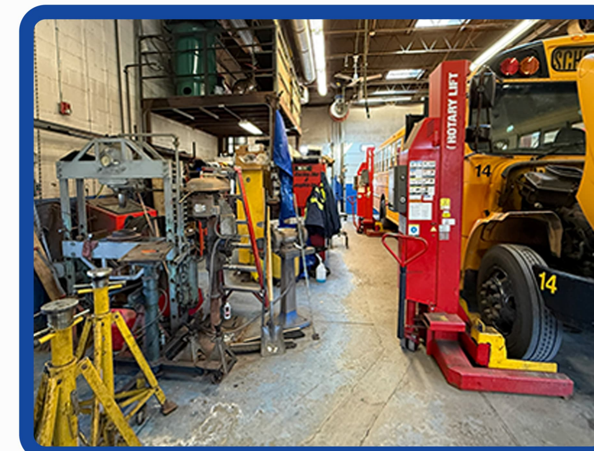
Unsafe Clearance for Personnel, Equipment & Buses
